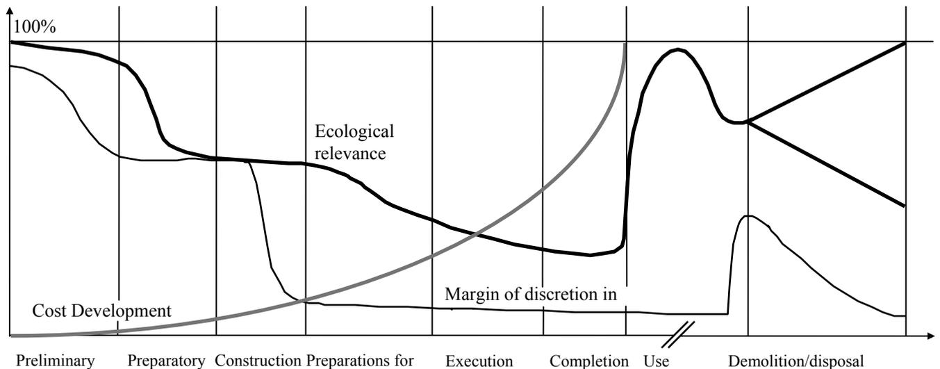
**Figure 1: Possibilities of influencing a building project; see text for explanations**
