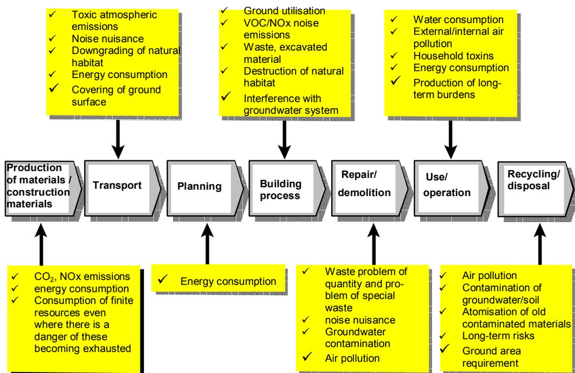
**Figure 2: Effects of constructions on the environment, from their manufacture to demolition**
