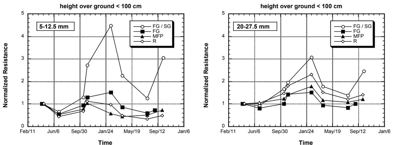
Fig. 6 Normalized concrete resistances over time measured with the instrumented cores at different depths
