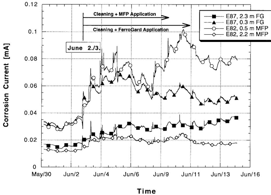
Fig. 3 Corrosion current of some electrically isolated rebars during the time of the cleaning process of the surface and the application of the inhibitors.
