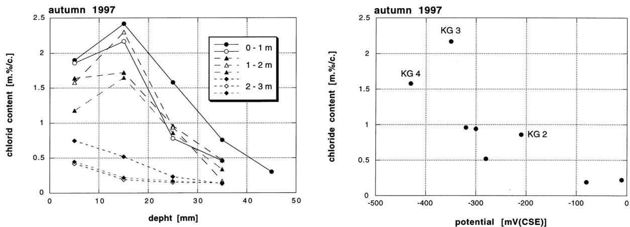
Fig. 1 Chloride profiles in different heights above ground and relation between chloride content and potential and corrosion state of the rebar in openings (KG: grade of corrosion) KG 0: blank, no corrosion / KG 1: slight signs of corrosion / KG 2: small areas with corrosion / KG 3: corrosion on the whole surface / KG 4: pitting corrosion
