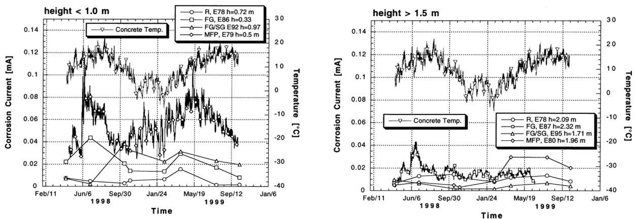
Fig. 4 Concrete temperature and corrosion current of some electrically isolated rebars of the differently treated test fields located at heights of <1.00 m and >1.50 m above ground, respectively
