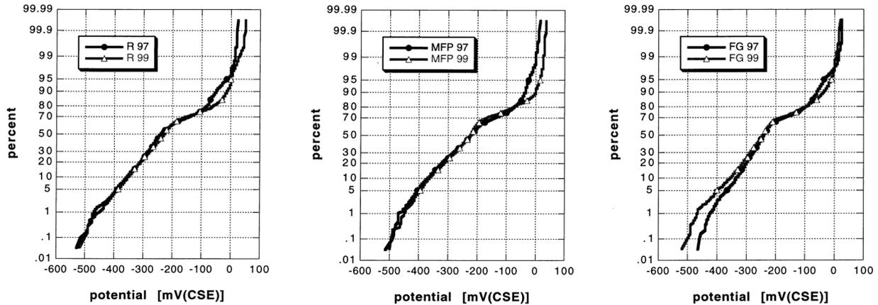
Fig. 2 Statistical analysis of the corrosion potentials measured 1997 and 1999 in the reference fields (R), the fields treated with MFP (MFP) and with FerroGard-903 (FG). 1997: Measurements before the application of the inhibitors 1999: app. 1.5 year after the application of the inhibitors
