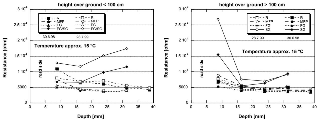
Fig. 7 Concrete resistances over the depth measured with the instrumented cores
