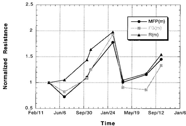
Fig. 5 Normalized concrete resistances (averages) over time measured with the electrically isolated rebars
