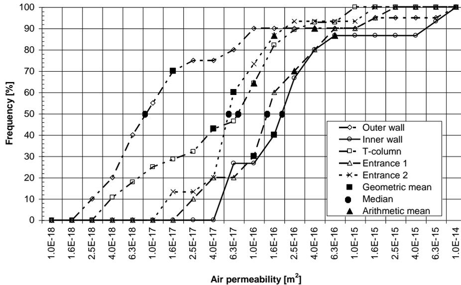
**Fig. 4: Cumulative frequency of air permeability values of different construction units; several mean values are marked: median, arithmetic geometric mean).**
