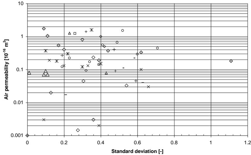
**Fig. 5: Mean air permeability versus standard deviation calculated without the extreme values**
