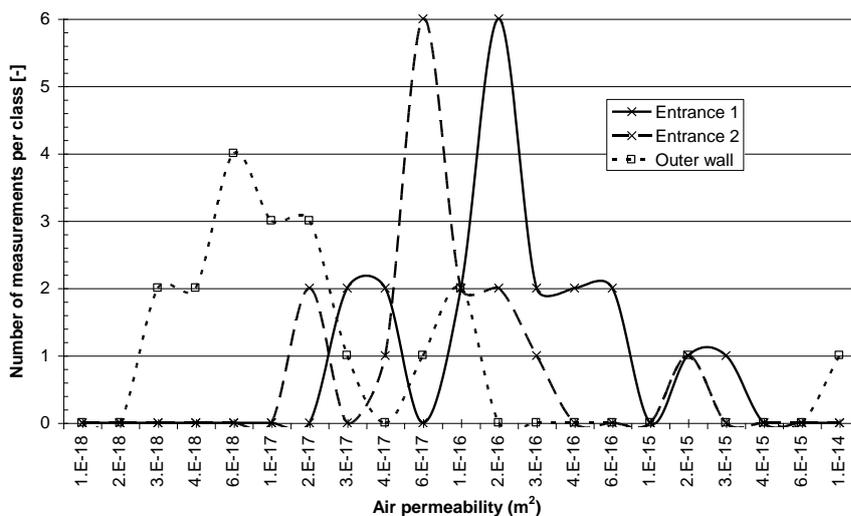
**Fig. 3: Distribution of air permeability values, determined on various structural members.**
