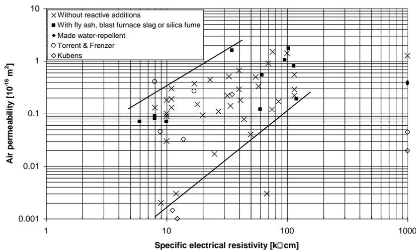
**Fig. 6: Mean air permeability (without extreme values) as function of specific electrical resistivity**
