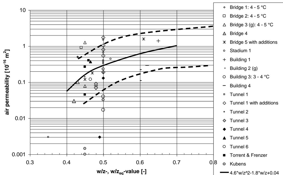
**Fig 7: Air permeability and w/c ratio; filled symbols: resistivity < 20 kΩcm; (g): w/c estimated from compressive strength. Air temperatures less than 5 °C are indicated in the legend.**
