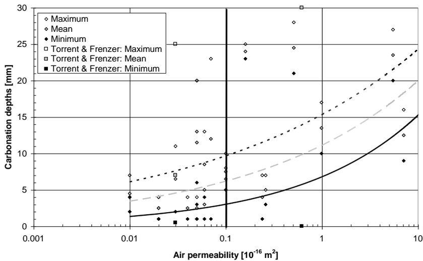
**Fig. 9: Carbonation depths as function of air permeability.**
