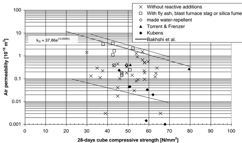
**Fig. 8: Mean air permeability (without extreme values) as function of the 28 days compressive strength; additionally the relationship from Bakhshi et al. [10] for laboratory concrete is shown.**
