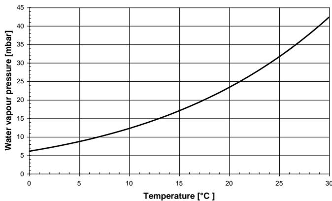
**Fig. 2: Water vapour pressure as function of temperature; data taken from Handbook of Chemistry and Physics.**
