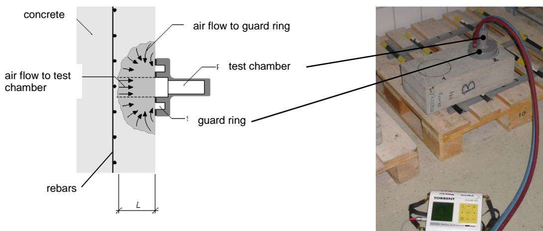
**Fig. 1: Left: sketch of the principle of the TPT-method (from SIA 262/1); right: measuring device on concrete specimen.**
