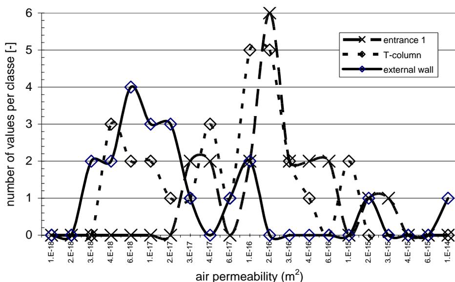
Figure 2: Results of air permeability measurements on different structural members
