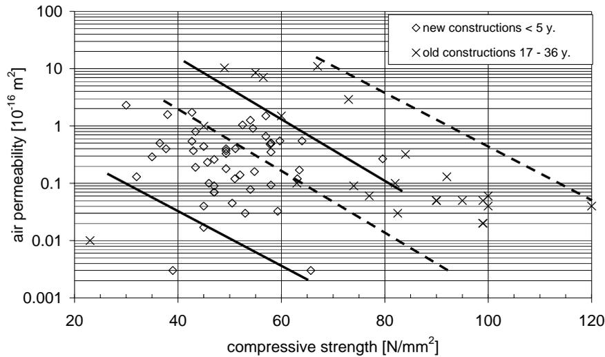
Figure 7: Results of air permeability measurements on site and compressive strength determined for new constructions on cubes having an age of 28 days and for old constructions on drilled cores (l = d = 50 mm).
