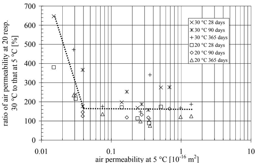
Figure 8: Influence of temperature and air permeability at 5 °C on air permeability measured at 20 and 30 °C.
