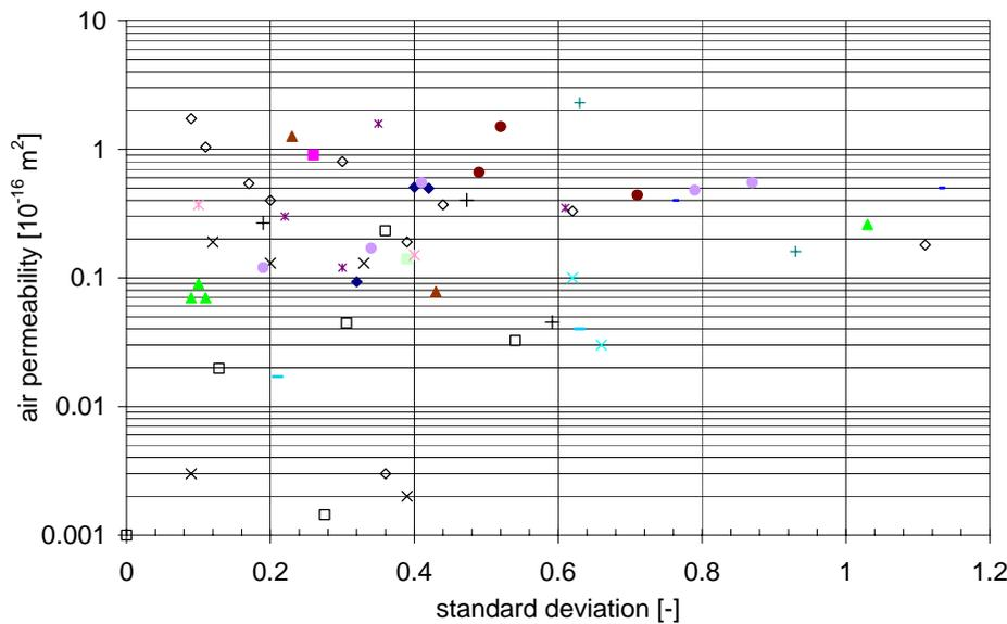
Figure 4: Standard deviation calculated from all measurements for each structural member as function of air permeability
