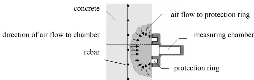
Figure 1: Sketch of the principle of TPT [6]
