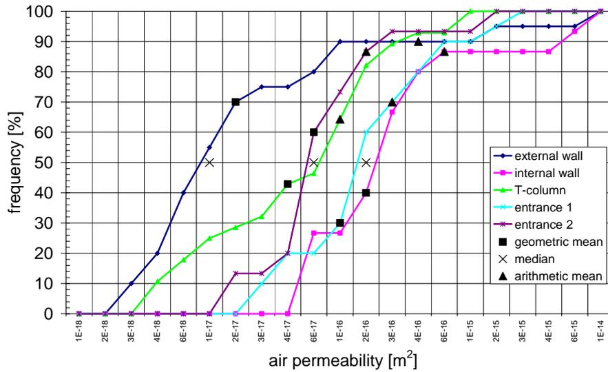
Figure 3: Distribution of air permeability values and various mean values for several structural members
