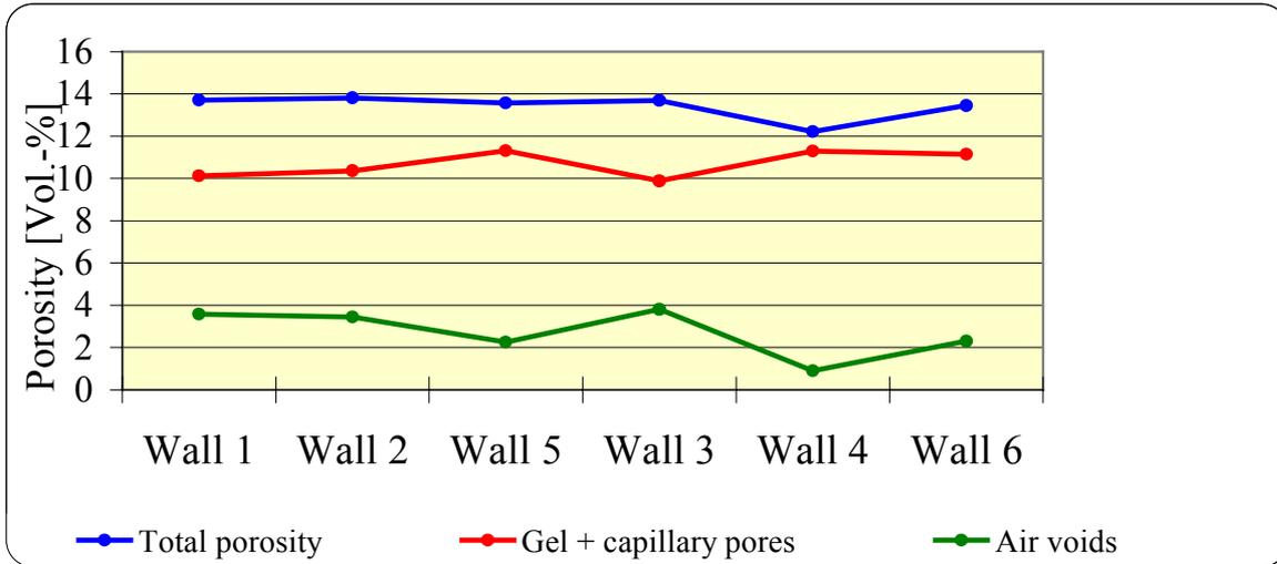
Fig. 4 Porosity of high-sand concrete mixtures, 0-32 mm, W/C ratio = 0.46, walls 3, 4 and 6 with steel fibers
