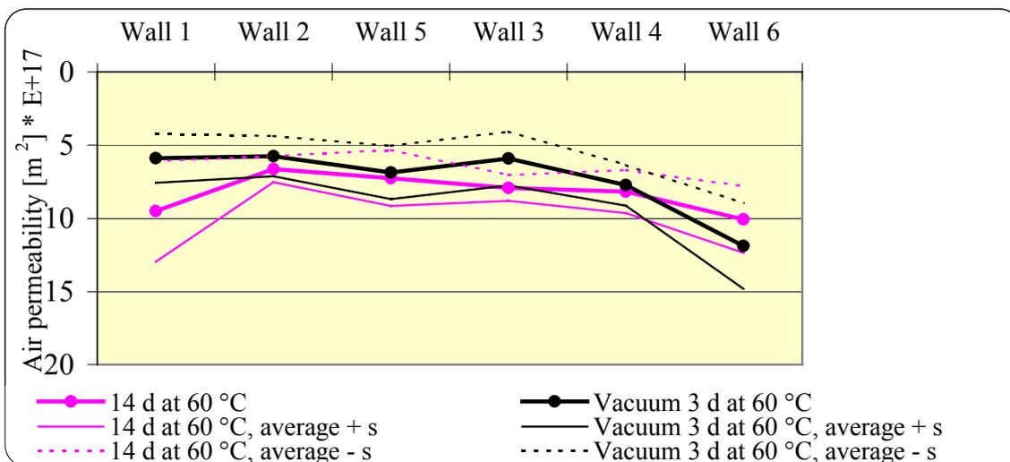
Fig. 5 Air permeability of high-sand concrete mixtures, 0-32 mm, W/C ratio = 0.46, walls 3, 4 and 6 with steel fibers, testing pressure = 1.5 bars
