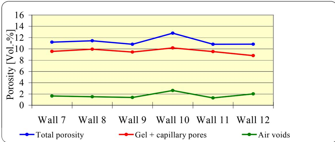
Fig. 6 Porosity of low-sand concrete mixtures, 0-32 mm, W/C ratio = 0.43, walls 10, 11 and 12 with steel fibers
