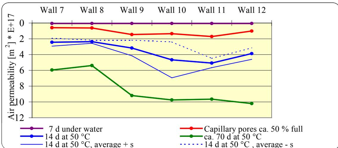
Fig. 7 Air permeability of low-sand concrete mixtures, 0-32 mm, W/C ratio = 0.43, walls 10, 11 and 12 with steel fibers, testing pressure = 1.5 bars
