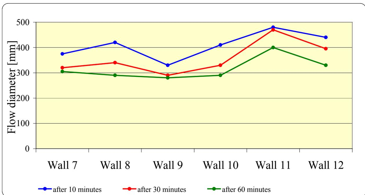
Fig. 3 Consistency of fresh concrete, wall 7 – wall 12
