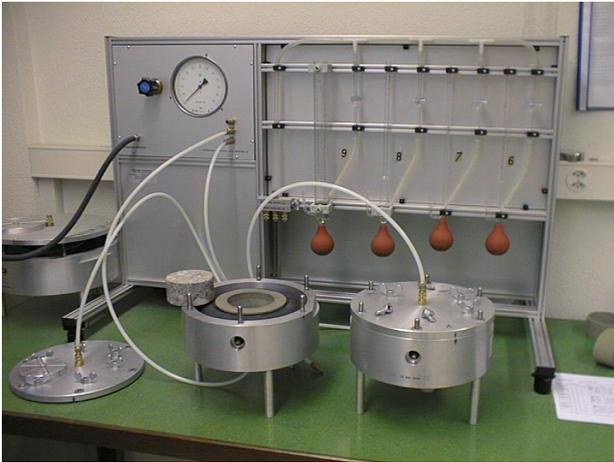
Fig. 2 Instrumentation used to determine air permeability
