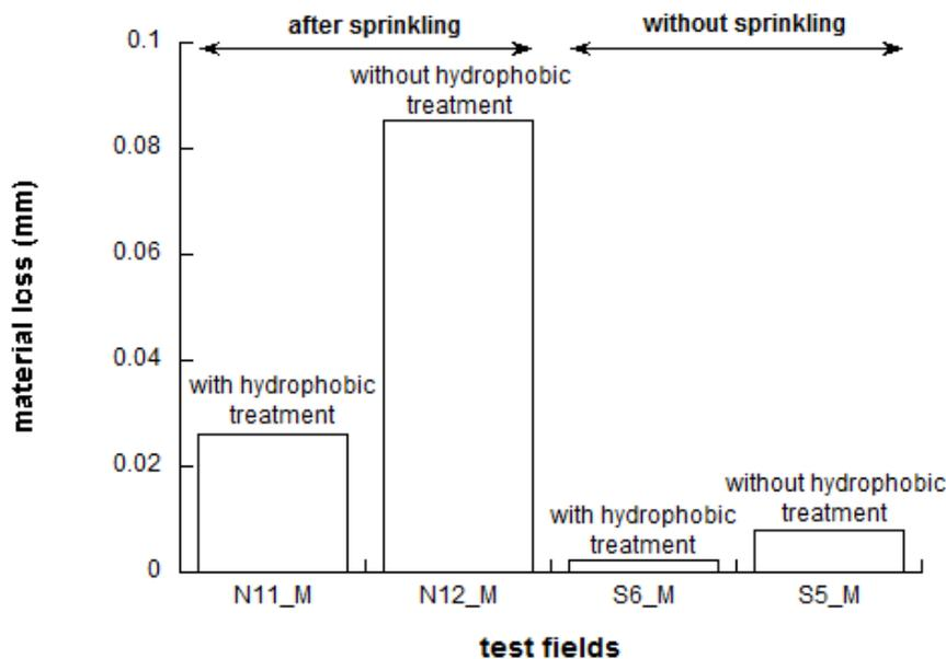
Fig. 3 Effectiveness of a hydrophobic treatment on the corrosion in a tunnel slab
