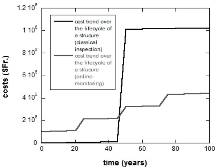
Fig. 2 Cost trend for the Lifecycle of a structure with or without using Online-Monitoring
