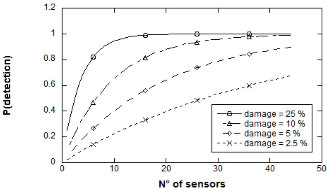
Fig. 1 Probability of detection at a certain damage level
